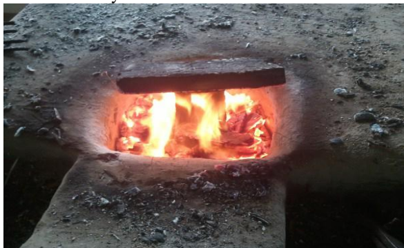
Fig.4 boiler tube heating in smithy furnace
