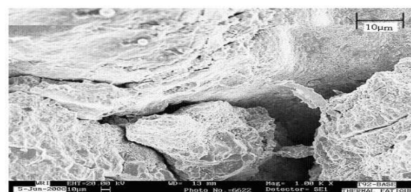
Fig.2 cracking along the grain boundaries
