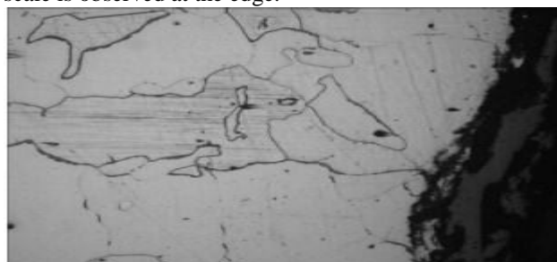
Fig.29 200 thermal cycles material of tube at internal side magnification of 400 X
